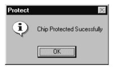
To protect the contents of flash memory, click <Protect> from the <Device> menu. The lock bits are properly programmed as per your requirement and the status is displayed in a small window.
